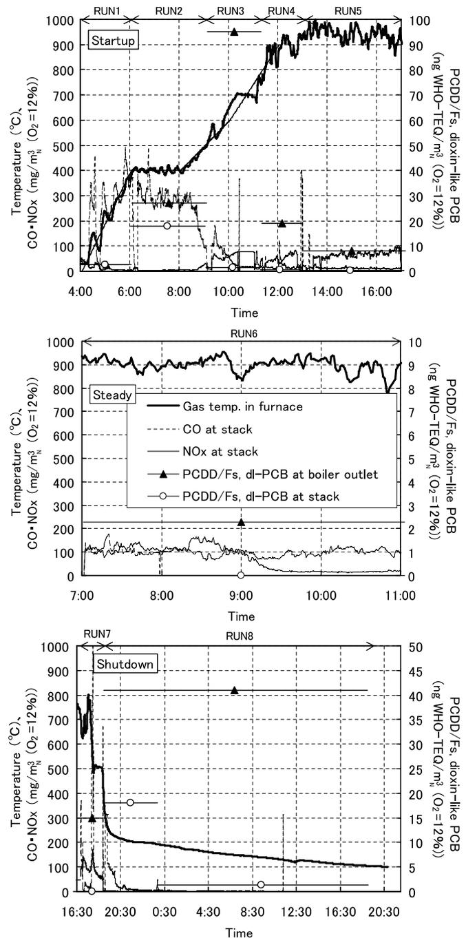
Fig. 3. Gas temperature inside the combustion chamber. CO and NO<sub>x</sub> concentrations at stack. PCDD/Fs, dioxin-like PCB concentrations at boiler outlet and stack.
