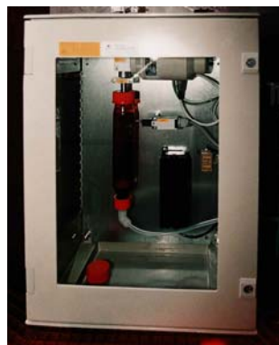
Cartridge box with XAD II cartridge
